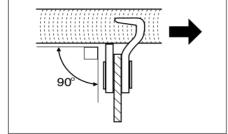
All cutters must be sharpened to the same angle, 30°. Different angles result in a roughly, irregularly running chain, increase wear and tear and cause chain beakage. The 85° front rake of the cutter results from the cut depth of the round file. If the proper file is used in the right manner, the correct front rake will be obtained automatically.
