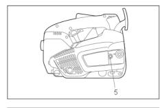
Turn the chain adjusting screw (5) to the left (counterclockwise) until the pin (6) is at the right stop.
